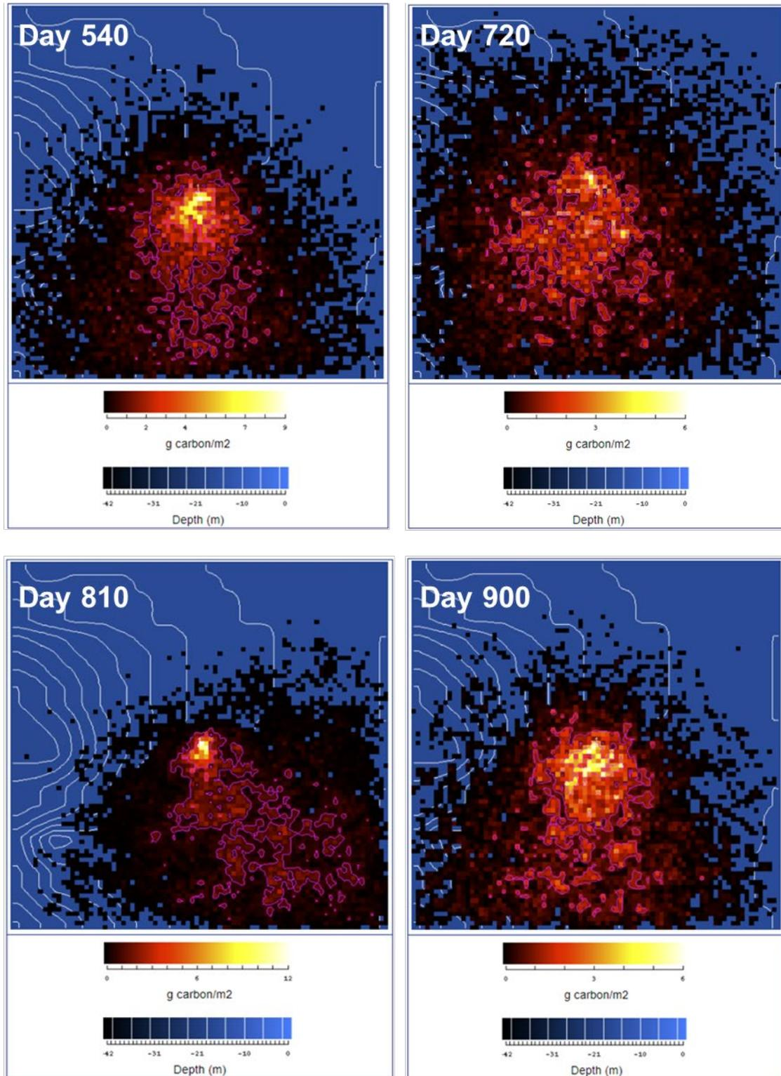
**Appendix:** Time-series simulation of predicted benthic carbon deposition beneath one net pen with a standing stock biomass of 36,288 kg of Almaco Jack (*Seriola rivoliana*). The reader should use caution comparing plots. The software generates a new legend for each plot in the time series. The scale and color ramp varies with each surface plot.
