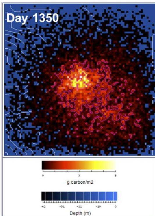
**Appendix:** Time-series simulation of predicted benthic carbon deposition beneath one net pen with a standing stock biomass of 36,288 kg of Almaco Jack (*Seriola rivoliiana*). The reader should use caution comparing plots. The software generates a new legend for each plot in the time series. The scale and color ramp varies with each surface plot.
