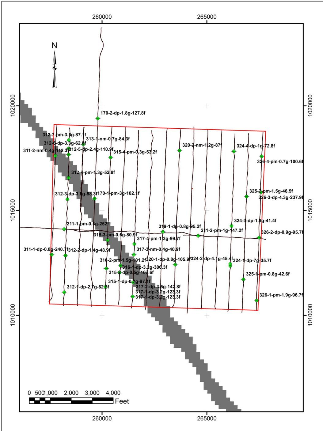
Figure 4. Location of magnetic anomalies in survey area.
