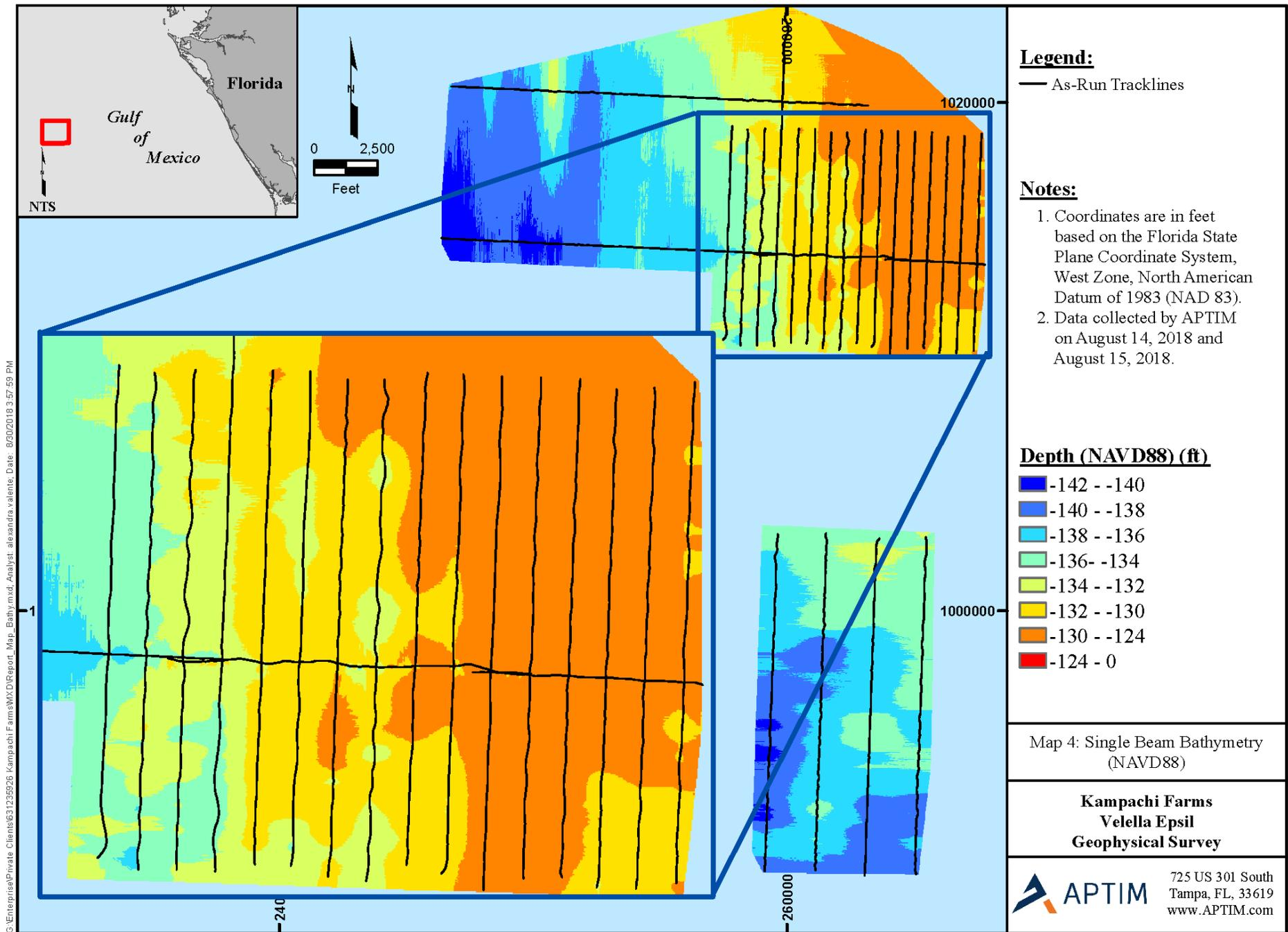
Figure 3. Single Beam Bathymetry Conducted at Modified Site B during the BES Fieldwork
