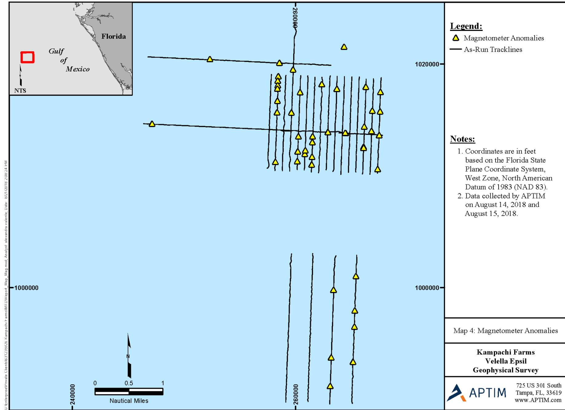
Figure 9. Magnetometer Anomalies Detected during BES Fieldwork (APTIM 2018)
