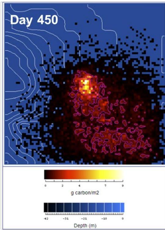
**Appendix:** Time-series simulation of predicted benthic carbon deposition beneath one net pen with a standing stock biomass of 36,288 kg of Almaco Jack (*Seriola rivoliana*). The reader should use caution comparing plots. The software generates a new legend for each plot in the time series. The scale and color ramp varies with each surface plot.
