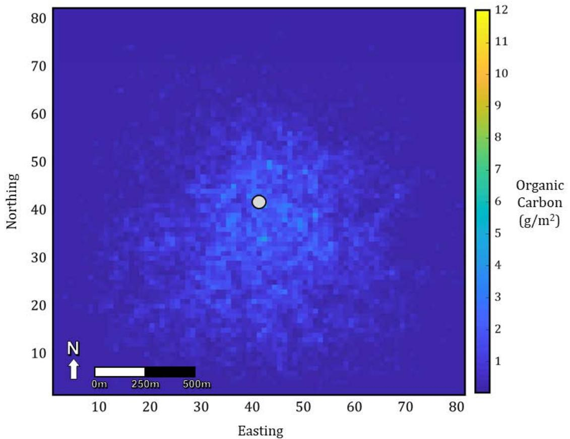
**Figure 3.** Predicted annual benthic carbon deposition field beneath one net pen with a standing stock biomass of 36,280 kg of Almaco Jack (*Seriola rivoliana*). Gray circle indicates center position of the net pen. Axes indicate simulation cell numbers and deposition mass is in grams.
