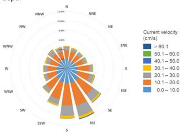
**Figure 2.** Distribution of current velocities (cm/s) and direction for NOAA Buoy Station 42022 located along the 50-m isobath approximately 45 miles northwest of project location. Currents are reported for water column depths of 4 m, 24 m, and 36 m.
