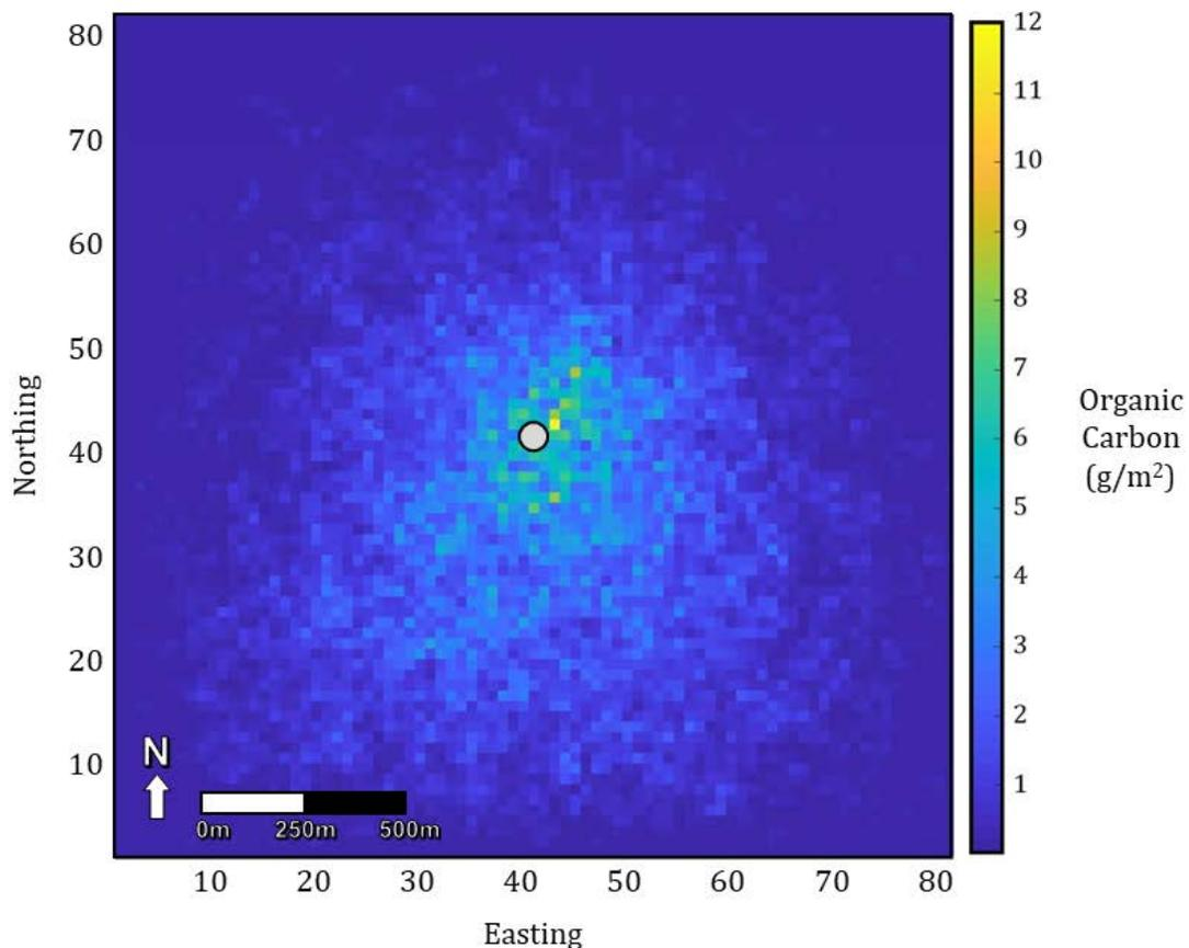
**Figure 4.** Predicted annual benthic carbon deposition field beneath two net pens with a standing stock biomass of 72,560 kg of Almaco Jack (*Seriola rivoliana*). Gray circle indicates center position of the net pen. Axes indicate simulation cell numbers and deposition mass is in grams. The center of the pens is located at (27.056275 N, -83.216743 W). Predicted carbon loading was derived from the 12-month time series relationship based on depositional flux with resuspension.
